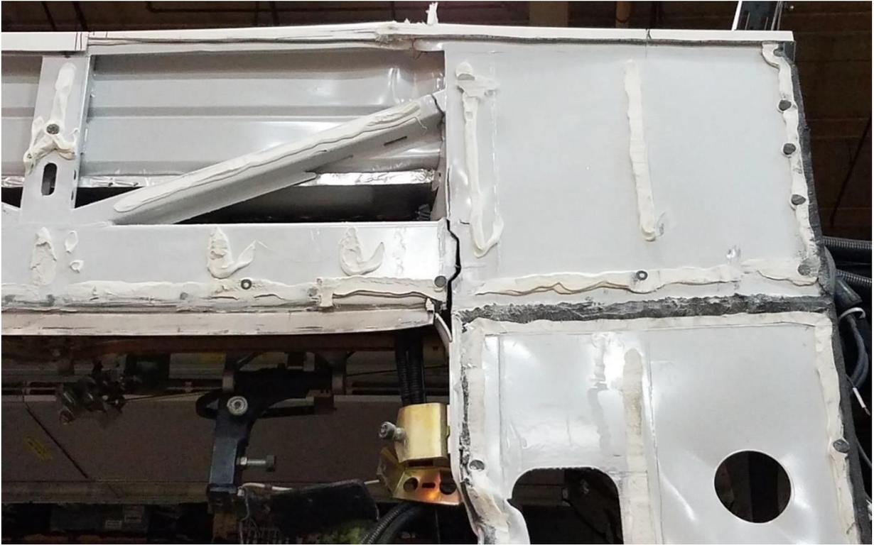
**Figure 25: A-Car LH Articulation Portal - Roof Support**
