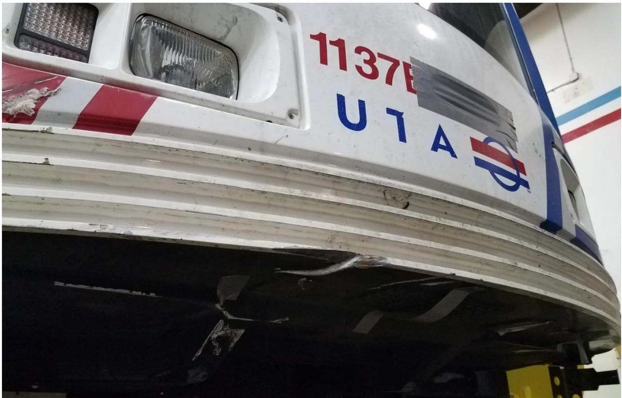
**Figure 33: B-Car Anti-Climber Damage**
