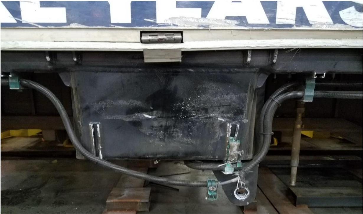
**Figure 34: C-Car Impact Side Damage**
