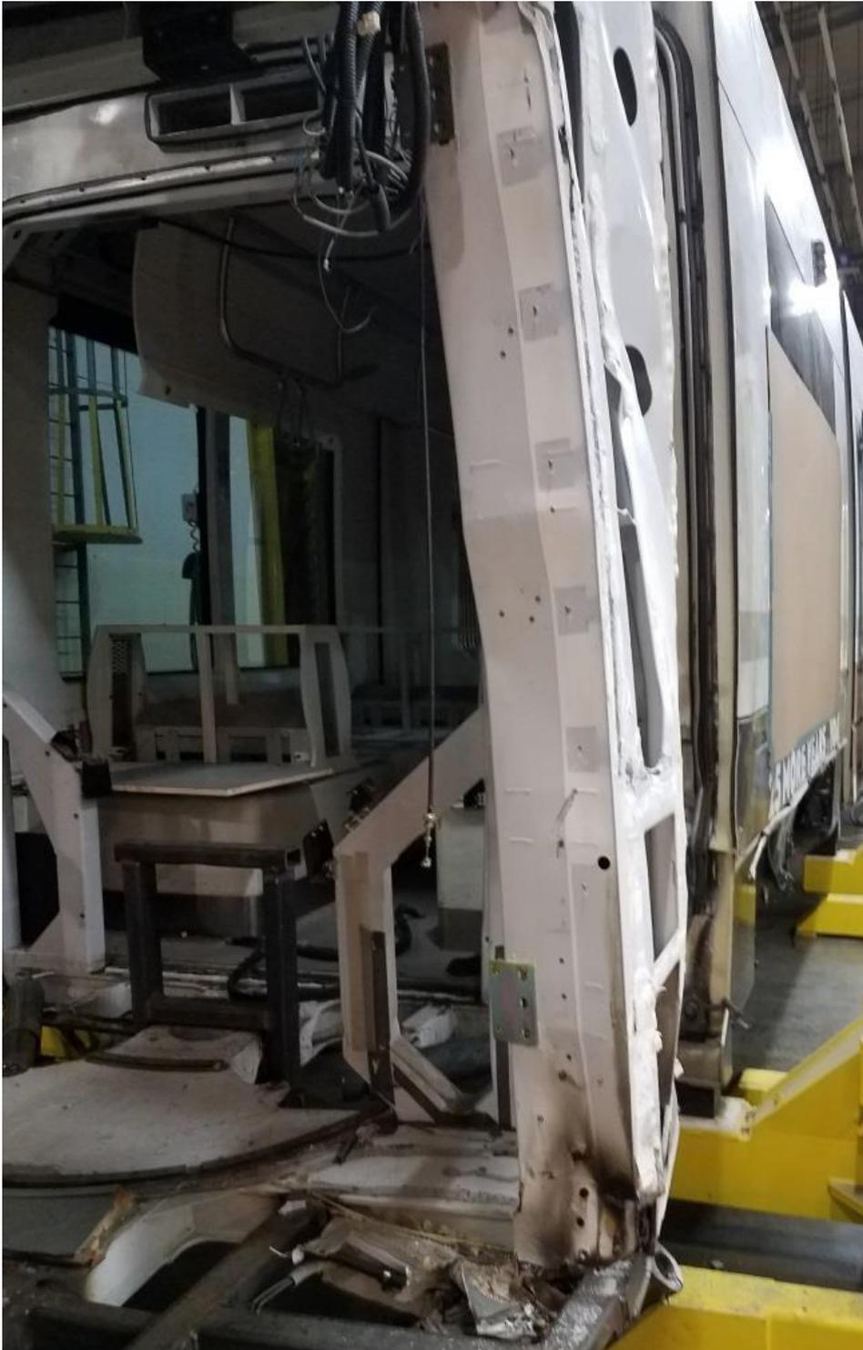
**Figure 24: A-Car LH Articulation Portal – Door Post View**
