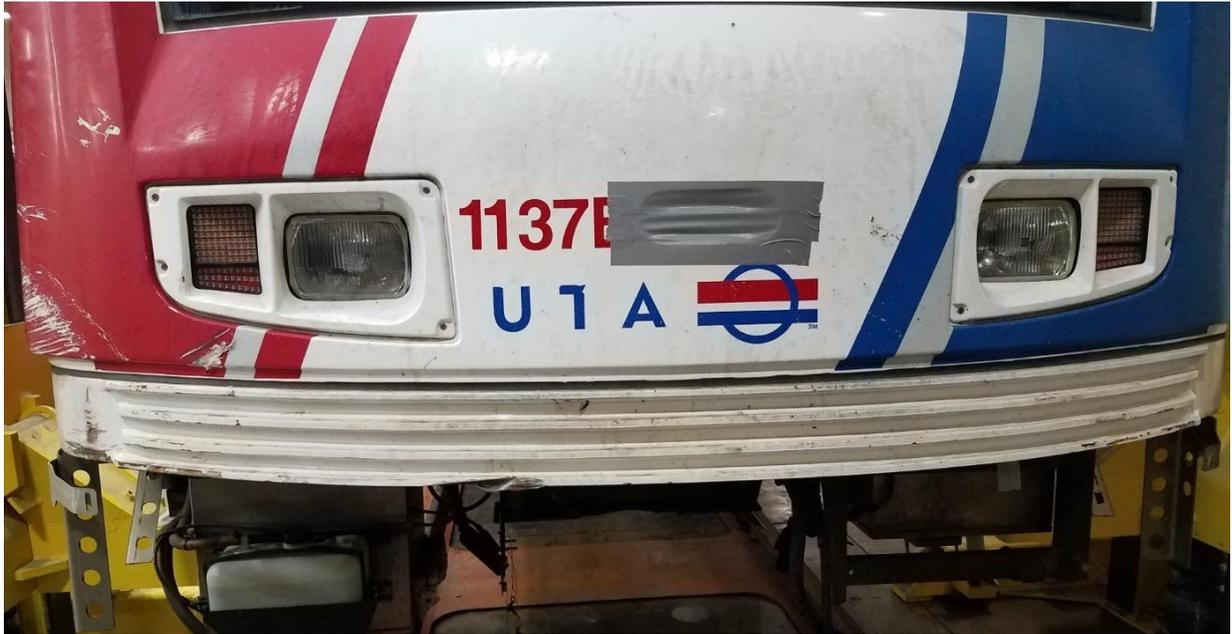
**Figure 32: B-Car Anti-Climber Damage**
